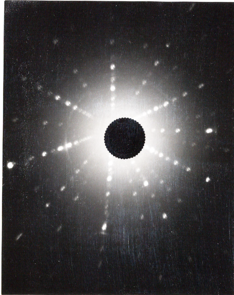
Figure 4d. Specimen 55R 1 , grain # 1 - omega Laue back-reflection photograph - near-perfect, but twinned structure re- flections from planes near (001). Cu target, 2 hour exposure, 25 mil pinhole, 3 cm. distance.
