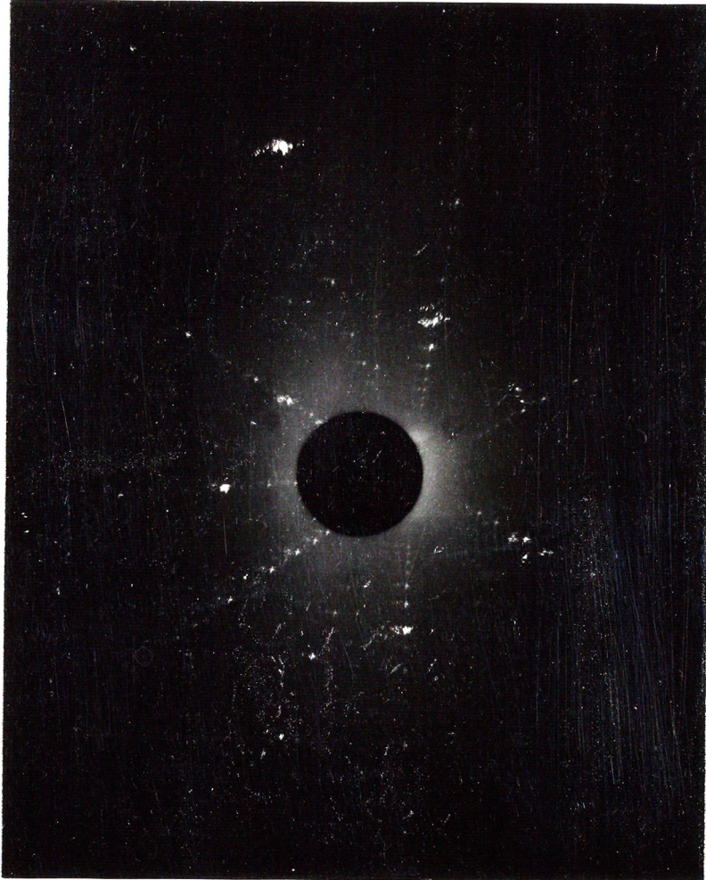
Figure 3c. Specimen 52 - alpha Laue back-reflection photogram - striated reflections from planes close to (001). Cu target, 2 hour exposure, 10 mil pinhole, 3 cm.
